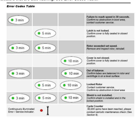
3) To clear the error condition, correct the problem and press the Stop/Open button.
