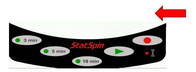
The cause of the error condition can be identified by the combination of green cycle time indicators that are also flashing. See Error Codes Table.
